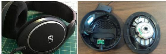
**Figure 1** Left: Sennheiser HD558 headphone. Right: The HD558 with speaker flange removed showing rear speaker and rear volume.
