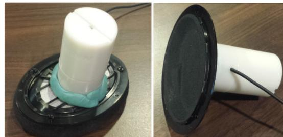
**Figure 3** Left: An MAE130 being used to measure the impedance  $Z_{fl\_spk} + (Z_{cushion} \parallel Z_{front\_vol} \parallel Z_{flange})$  seen by the front of the speaker. The cushion is on a rigid table surface, so  $Z_{load}$  is infinite in this case. Right: The MAE130 being used to measure  $Z_{fl\_spk}$ .
